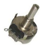
380 Series Industrial Potentiometer, Conductive Plastic Element, Solder lug Terminals, 2 W Power Rating, 500 kOhm Resistance Value
